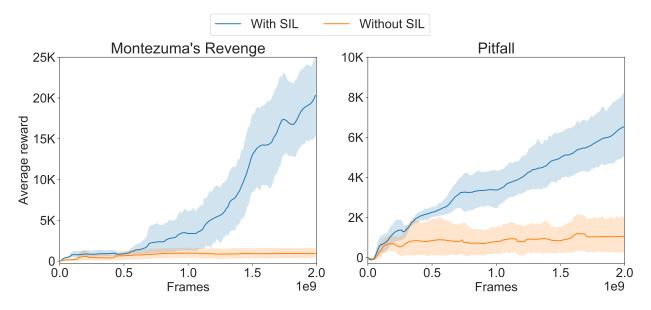
Supplementary Figure 8: Policy-based Go-Explore with and without the Self Imitation Learning (SIL) loss. The SIL loss provides substantial increases in terms of average score on both Montezuma's Revenge and Pitfall. Shaded areas show 95% bootstrapped confidence intervals of the mean with 1,000 samples. Each line is averaged over 10 runs with independent seeds.
